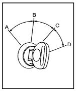
The ignition switch has four different positions.
